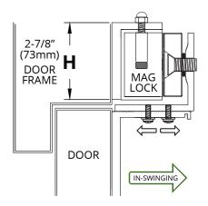
This professional grade LZ bracket is finished in anodized aluminum. It is the perfect solution for installing magnetic locks on In-Swinging Doors.
